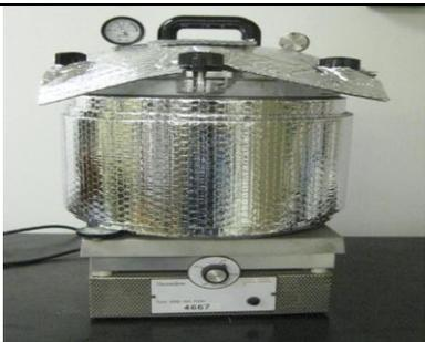
**Autoclave test** is to evaluate water immersion resistance at a **temperature** above boiling point. It is a good screening tool to evaluate coating performance in hot water.
