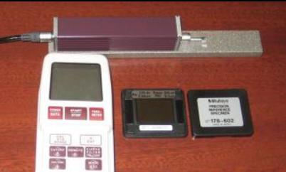
**Mitutoyo SJ-201 Surface Roughness Tester**, measures the surface profile. Surface roughness parameters, such as Rz, Ry, Sm, Peak count, Pc can be displayed.
