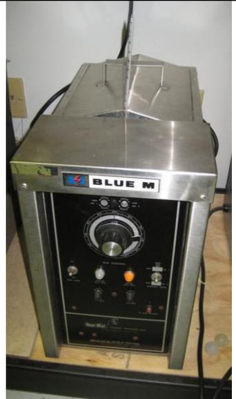
**Water Bath** is used to measure water absorption of polymers and coatings at temperature below boiling point.
