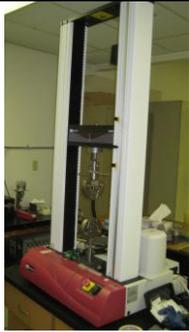
**Instron Testing Machine, Model # 3369** is a widely used mechanical testing machine to measure material tensile, compression, shear and flexure properties, such as strength, modulus, strain. It is controlled by Bluehill software and also equipped with accessories to measure Poisson ratio, peel strength coefficient of friction. A temperature chamber is also equipped to measure material properties at elevated temperatures.
