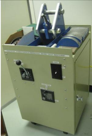
**Fixed Radii Mandrel Bending Machine** measures the flexibility of coatings applied on metal substrates. It gives very repeatable flexural strain measurements.
