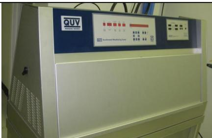
**QUV Chamber** (ASTM G154, D5894) examines the UV resistance of polymers/coatings. It can also cycle UV(shine) and water condensation (dark) to simulate atmospheric exposure.
