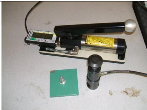
**PosiTest® Pull-Off Adhesion Tester, ASTM D4541,** measures tensile pull-off adhesion strength of coatings on metal substrates.
