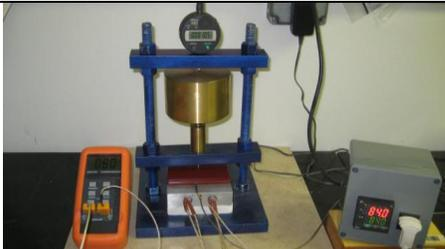
**The Penetration Resistance tester (ASTM G17)** measures the penetration resistance of buried pipeline coatings from rocks under soil pressure. A hot plate is used to heat coatings.
