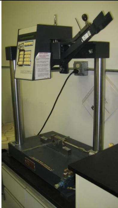
**Pendulum Impact Tester**, ASTM D256, measures the impact strength of notched polymers (Izod pendulum impact test).
