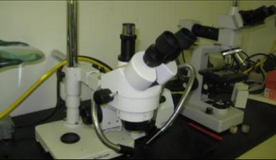
**Optical Microscopes** are used to examine coating material microstructure for failure analysis.
