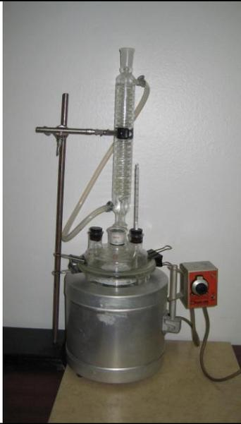
**Boiling Water Test** measures water absorption of coating samples at the water boiling temperature.
