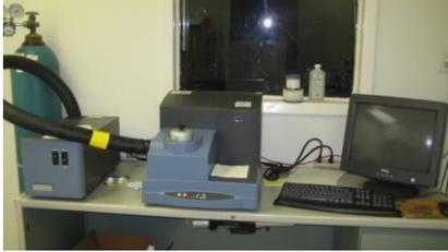
**TA Q20 DSC** measures thermal properties of polymers/coatings. such as glass transition temperature, melting point, crystallization temperature, degree of cure, oxidation induction time.
