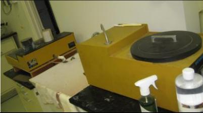
**Grinding/Polishing Wheels** are used to prepare samples for microstructure examination. It is a powerful tool for failure analysis.
