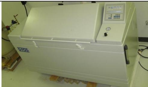
**QFog Salt Fog (Salt Spray) test Chamber** (ASTM B117, D5894, G85) examines the corrosion resistance of protective coatings.
