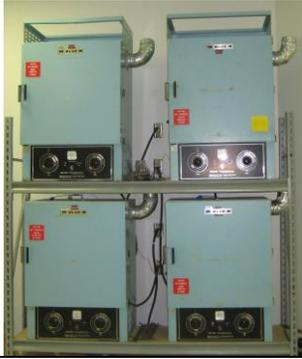
**Constant Temperature Ovens** are used to conduct long term thermo-oxidative aging of polymers/coatings.
