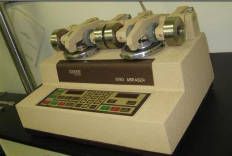
**Taber Abraser, ASTM D4060,** measures abrasion resistance of polymers / coatings
