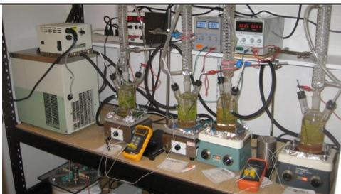
**Cathodic Disbondment tester** (ASTM G8, G42, G95, D6676) measures coatings' resistance to disbonding, imposed by cathodic protection current. High temperature testing capabilities are also equipped to test cathodic disbondment at high temperatures.
